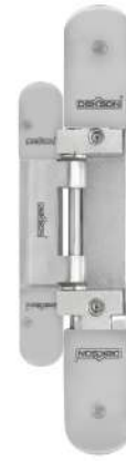
CONCEALED HINGE ESS CONC D100 SSS Capacity (max) : 100 KG / pair Max. Door Width: 100 cm Opening Angle : ≤ 150°
