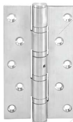
NRP ESS 316 6X3,5X4MM 4BB SSS Capacity (max) : 100 KG / pair
