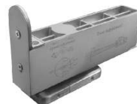
DPH 0980 NA Capacity (max) : 80 Kg Door Width : 800 - 950 mm Door Thickness (min) : 45 mm Suitable For Indoor Use * Accessories FH Top Pivot to be ordered separately
