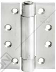
SPRING HINGE ESS SPR 4X3X3MM SSS Available : 4X4X3MM SSS Capacity (max) : 30 KG / pair Max Door Widht : 80 cm (Not suitable to be applied to hotel lock doors)
