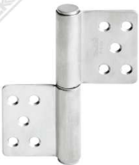
FLAG HINGE ESS FH 127X63X3MM 1W SSS Capacity (max) : 50 kg / pair
