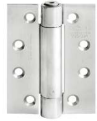
SPRING HINGE ESS SPR 4X3X3MM SSS Available : 4X4X3MM SSS Capacity (max) : 30 kg / pair Max Door Widht : 80 cm (Not suitable to be applied to hotel lock doors)
